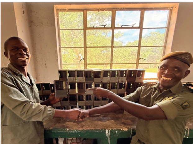
Custom metal housings to protect Bushnell camera traps from elephants and hyenas. More than eighty units ready for grid deployment across the park to assess wildlife populations.
